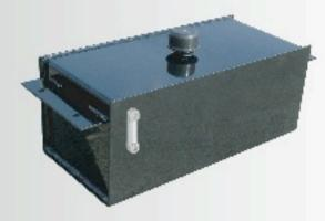
The 8.5 gallon box type reservoir is designed to be frame mounted. It hangs out of the way and is equipped with a brass wire mesh suction strainer, oil level & temperature gauge.
